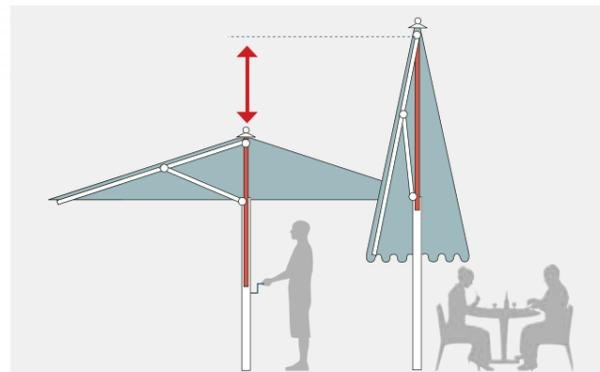
When the shade closes, the telescopic system elongates the mast. The advantage – There's no need to remove seating or tables beforehand.
